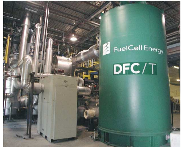
Fig. 7. Stack FA-100-2 test in 400 kW-class power plant: DFC ® /T proof-of-concept and stack design demonstration.
